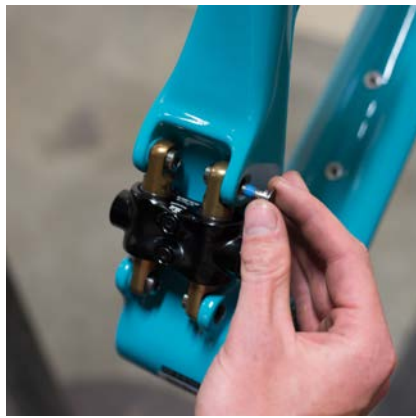
08. Prep 4X Flat Head Ti Male bolts (300030156) with blue Loctite. Install a Flat Head Male Ti Bolt through the Front Triangle into the Ti Female Bolts. Repeat for all four locations
