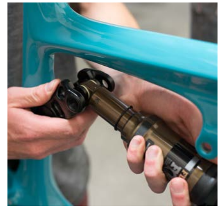
12. Install the rear shock eyelet into the Link. Make sure that the shock controls are facing downwards, and secure with guide pins (note they will not pass through the frame).
