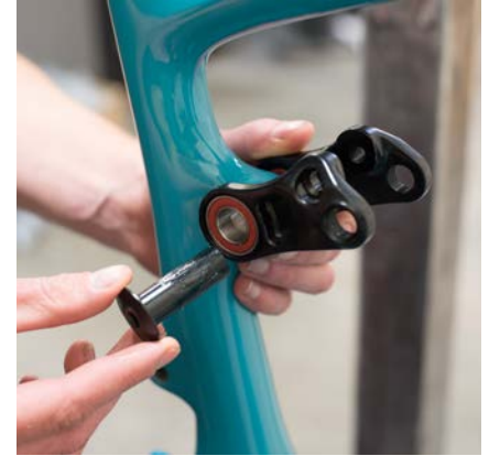
10. Apply a light coat of grease to the shaft of the Female Link Pivot Bolt (300030292). Slide the Alloy Link onto the Front Triangle and install the Female Link Pivot Bolt.
