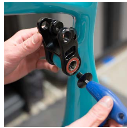
11. Grease the threads of the Male Link Pivot Bolt (300030293). Install into Female Link Pivot Bolt.
